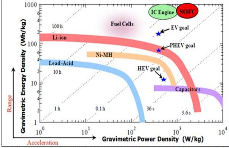
Legend: solid oxide fuel cell (SOFC); internal combustion (IC) engine; nickel-metal hydride battery (Ni-MH); hybrid-electric vehicles (HEV); electric vehicles (EV); and plug-in hybrid-electric vehicles (PHEV).
